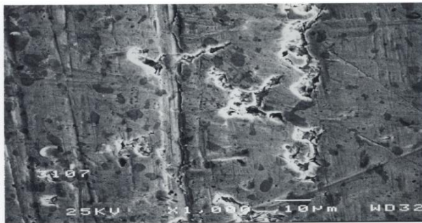
Figure 2: Lead-tin-copper overlay fatigue
